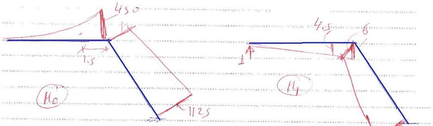
$$\Delta_{B0} = -\frac{1}{EI} \left[ \frac{1}{3} \times 450 \times 6 \times 4.5 \right] - \frac{75}{EI} \left[ \frac{450 \times 6 + 1125 \times 10.5}{3} + \frac{450 \times 10.5 + 1125 \times 6}{6} \right]$$
