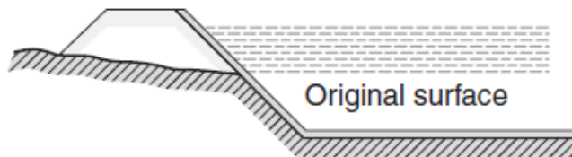
(c) Open service reservoir
