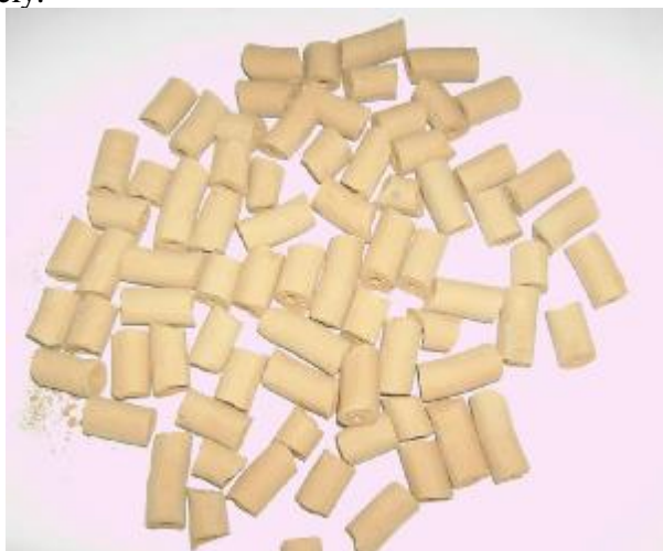
Fig. 1. Fractions of silver and molybdenum catalyst ZB-Ag_2O , Al_2O_3-MoO_3-Ag_2O
