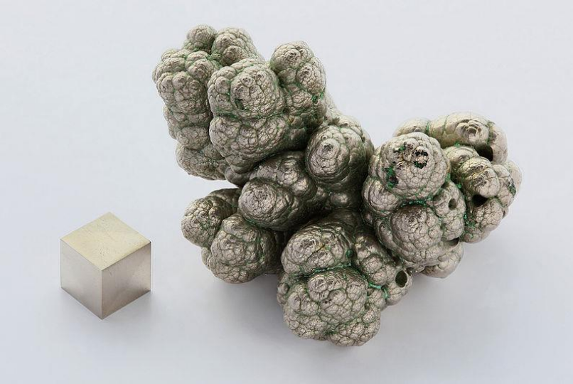
Electrolytically refined nickel nodule , with green, crystallized nickel-electrolyte salts visible in the pores.
