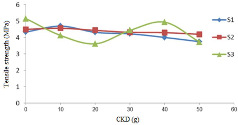
**Fig. 5. Effect of adding CKD on tensile strength of the pastes.**
