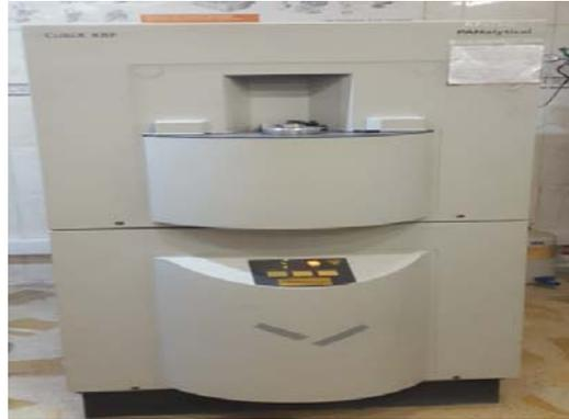
**Fig. 12. X-ray fluorescence device**
