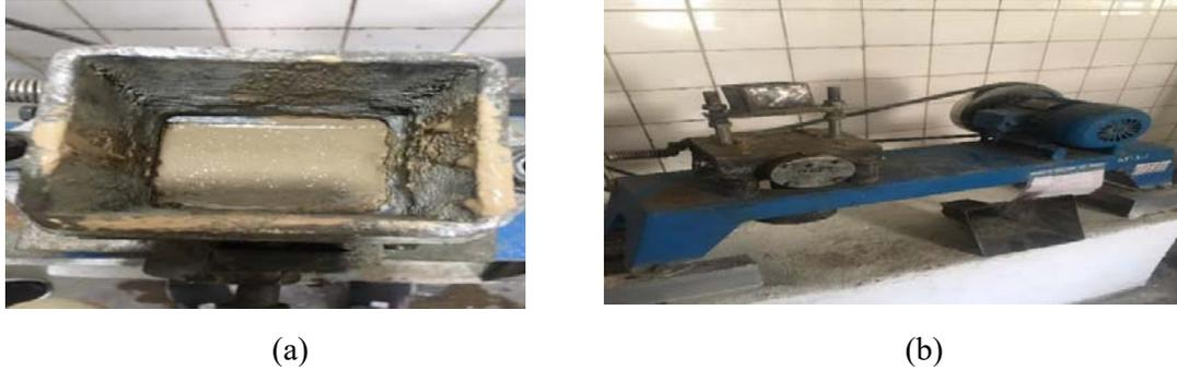
**Fig. 3. (a) Mixing device of CKD and RO water; (b) vibration detecting device.**
