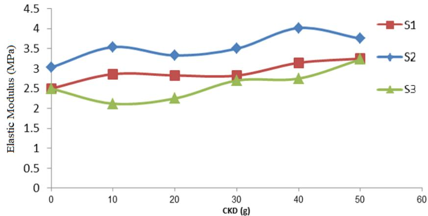
**Fig. 8. Effect of adding CKD on the elastic modulus of the pastes.**
