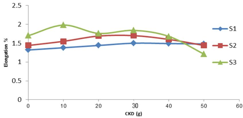
**Fig. 6. Effect of adding CKD on elongation of the pastes.**
