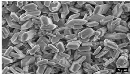
**Fig. 7. A microscopic photograph of the paste with 40 g CKD**
