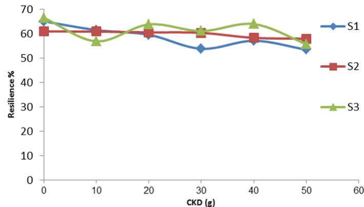
**Fig. 9. Effect of CKD additive on the resilience of the pastes.**
