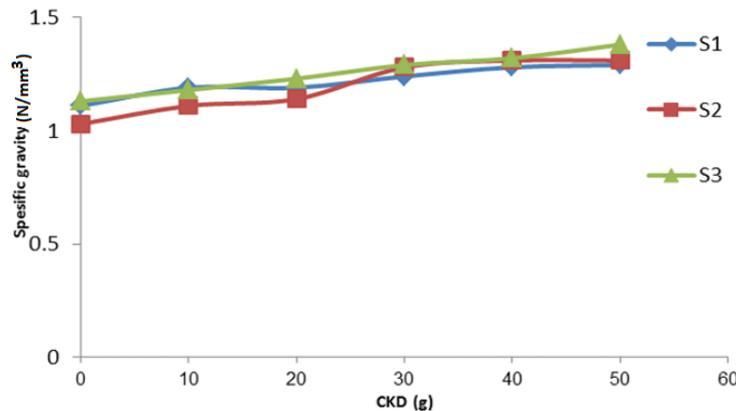
**Fig. 11. Effect of CKD additive on the specific weight of the pastes.**
