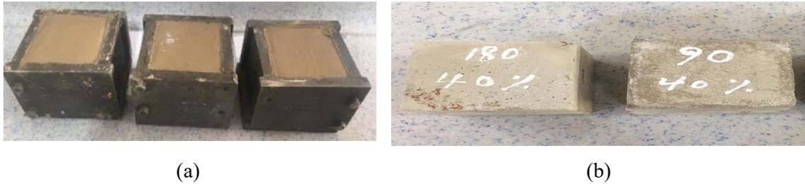
**Fig. 4. (a) Specimens after mixing inside the moulds; (b) specimens after drying.**
