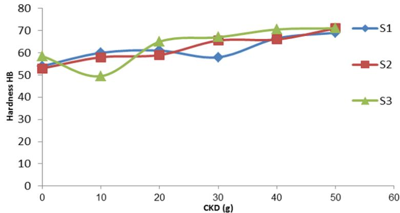
**Fig. 10. Effect of CKD additive on the hardness of pastes.**
