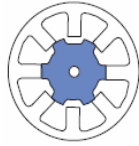
4- phase , 6 rotor poles, 8 stator poles
