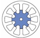
5- phase, 8 rotor poles 10 stator poles
