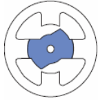
2- phase, 2 rotor poles 4 stator poles
