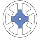
3- phase, 4 rotor poles 6 stator poles
